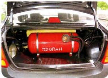
MOTORCAR WITH CNG EQUIPMENT
